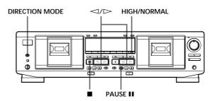
1 Insert a recorded cassette into deck A and a blank cassette into deck B.
